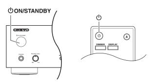
To turn on the CD Player, press the [ $\bigcirc$  ON/STANDBY] button on the unit or the remote controller. Press the [ $\bigcirc$  ON/STANDBY] button again to set the CD Player to Standby.
