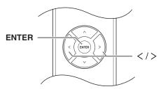
You can specify that if the CD Player is left stopped for 30 minutes, the power will automatically turn off, placing the unit in Standby mode (Auto Standby function).
